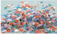
Racks are ground into small pieces
